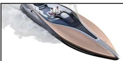
The Lexus of boats: We're not joking. This impossibly luxurious seacraft is the recently unveiled Lexus Sport Yacht, which is powered by two of the same V-8 engines found in the marque's RC F coupe. The exterior is made from carbon-fiber-reinforced plastic, just like its sportscar brethren. It's a one-off concept (meaning it's not for sale), but parent company Toyota does manufacture boats, so seeing your next Bond villain in one isn't a complete maritime fantasy. lexus.com
